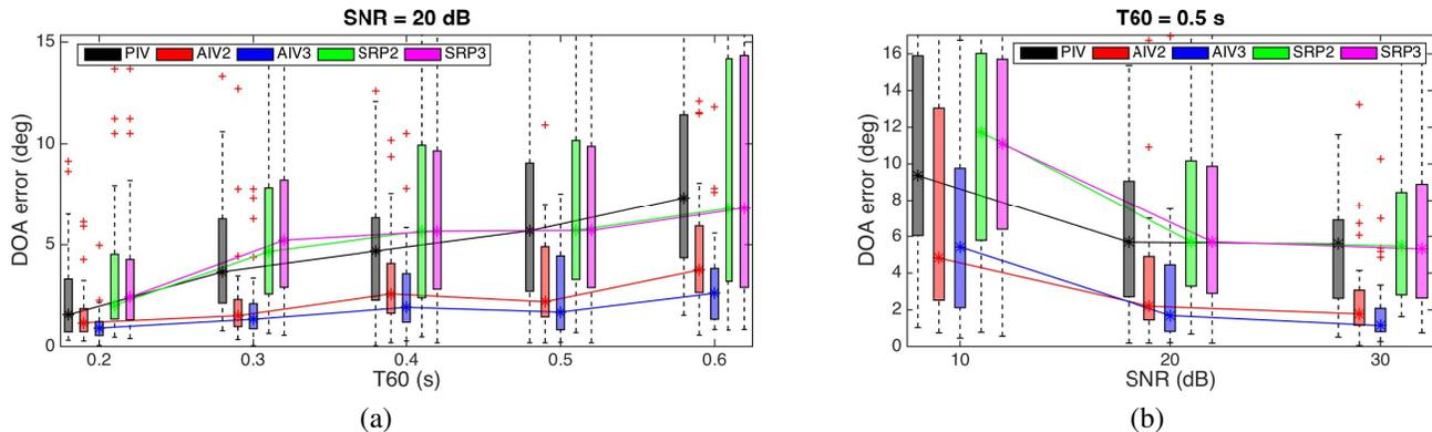
**Fig. 1.** The DOA errors for the PIV (black), second-order AIV (red), third-order AIV (blue), second-order SRP (green) and third-order SRP (magenta) as a function of reverberation time (a) and sensor noise level (b). The boxes show the median as an asterisk, upper and lower quartiles, and the whiskers extend to 1.5 times the interquartile range.
